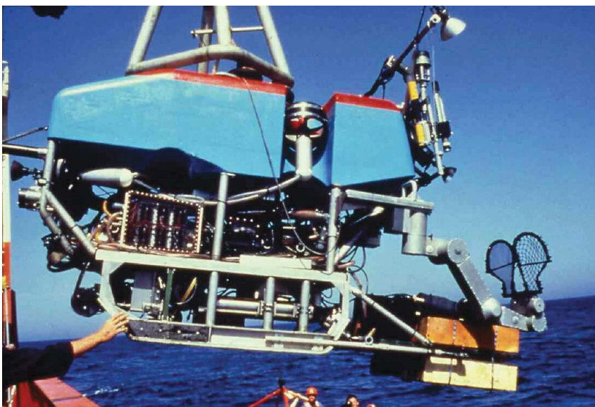
The Jason: remotely operated submersible with robotic manipulator (1997).
